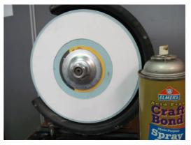
Adhere the paper disc to the outboard side of the wheel using photo mount spray.
