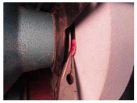
Installing sticky dots on the inboard side of the wheel using needle nose pliers.
