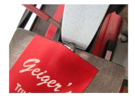
Traverse the Tru-N-Dress back and forth 6 to 8 times and then slightly advance the position of the diamond again (about 1/16<sup>th</sup> of a turn). Repeat this procedure a few times then stop the grinder and inspect the wheel. Repeat as necessary until it appears that the diamond has contacted the entire circumference and width of the wheel. Repeat the same procedures on the other wheel.
